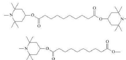
**GC UV LS 765** is a highly effective hindered amine light stabilizer (HALS). **GC UV LS 765** is in liquid form hence easy to incorporate and has low volatility and thermal stability. **GC UV LS 765** is applicable in a wide range of polymers including polyurethanes, sealants, adhesives, elastomers, unsaturated polyesters, acrylics, vinyl polymers (PVB, PVC), styrene homo- and copolymers, polyolefins, liquid color concentrates and other organic substrates.
