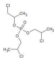
**GC TCPP** is a flame retardant used primarily in both rigid and flexible polyurethane foams, PVC, EVA, phenolics and epoxy resins. **GC TCPP** can be added at various points in polyurethane production: either in the production of foams or in the formulation of polyols to modify their viscosity.
